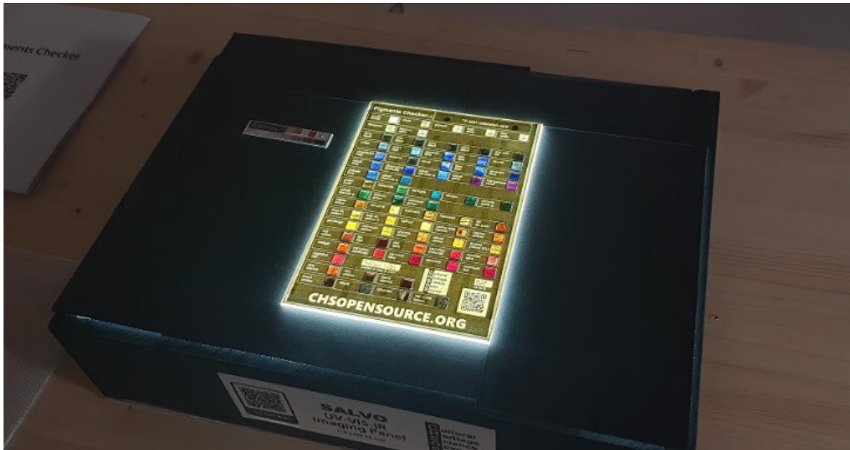
Figure [2]. Pigments Checker positioned on the SALVO Imaging Panel with black cardboard pieces used as screens. VIS LEDs are turned on.
