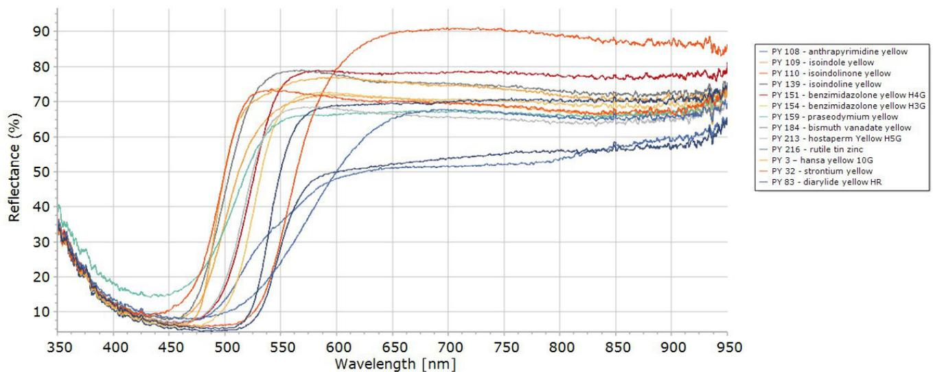
Figure 6. Reflectance spectra of the yellow pigments in Pigments Checker “Modern & contemporary Art”.
