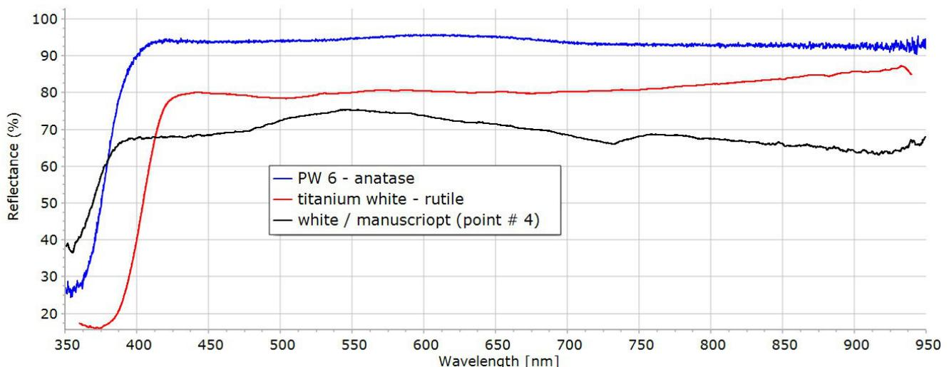
Figure 3. Reflectance spectra of the two types of titanium white, anatase and rutile, and of the white paint on a Indian Mughal manuscript.
