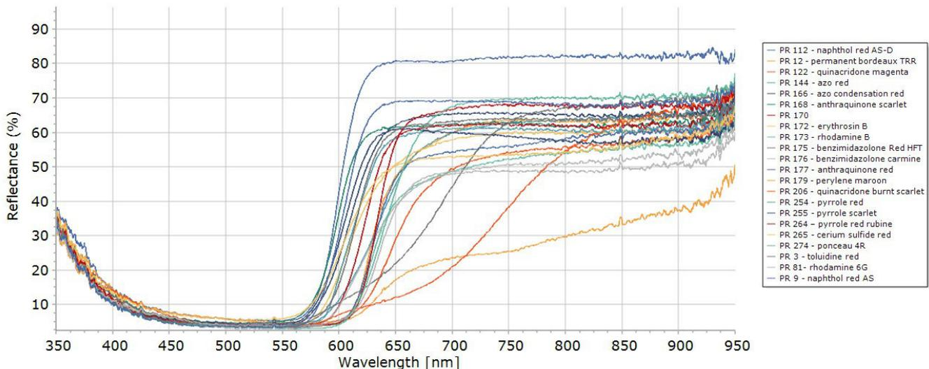
Figure 5. Reflectance spectra of the red pigments in Pigments Checker "Modern & contemporary Art".
