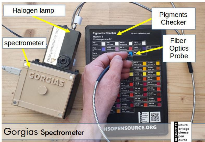
Figure 1. Gorgias Spectrometer testing on Pigments Checker "Modern & Contemporary Art".
