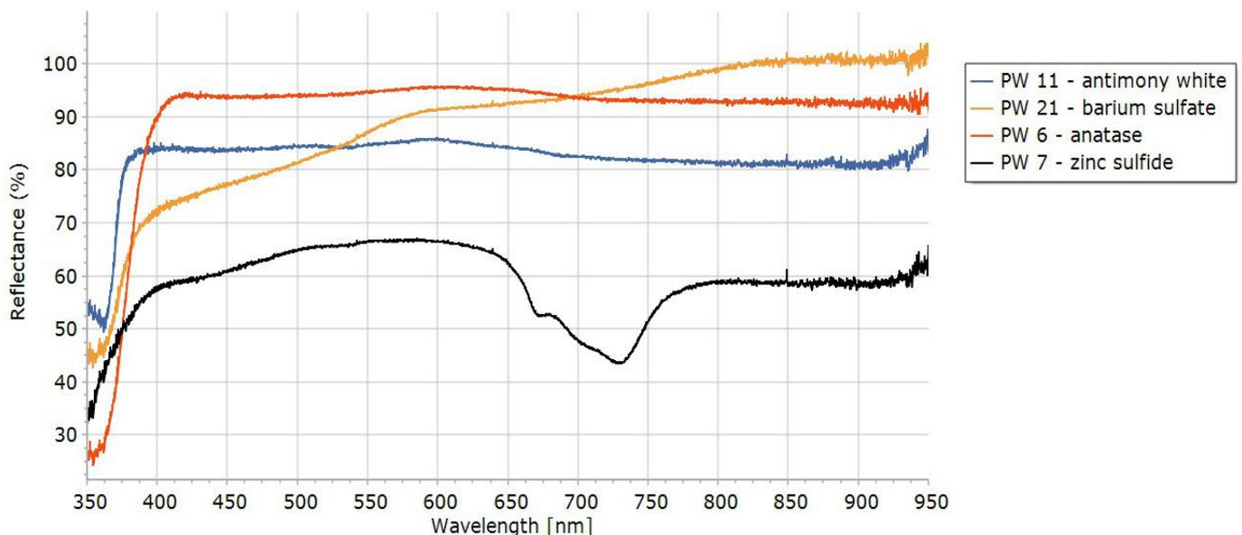
Figure 7. Reflectance spectra of the white pigments in Pigments Checker “Modern & contemporary Art”.
