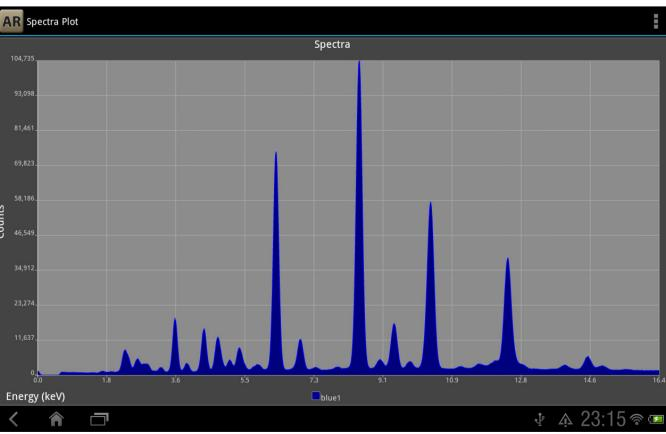
Figure 5. Example of spectra information for a blue pigment sample that can be accessed interactively, while the physical wood panel is being investigated.
