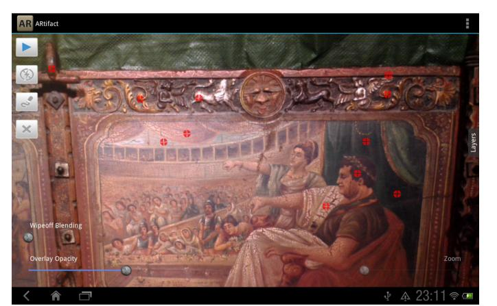
Figure 4. Augmented reality overlay, showing a video seethrough representation of a wood panel, augmented with cross-hair markers that are identifying where spectral data was collected.
