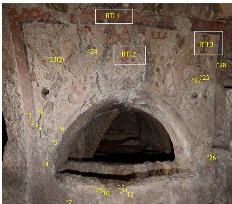
**Fig. 3.** Map of the spots analyzed with XRF spectroscopy on the “Deodata” mural painting. Reflectance Transformation Imaging (RTI) was also carried out, white box areas, in a subsequent study (in preparation).
