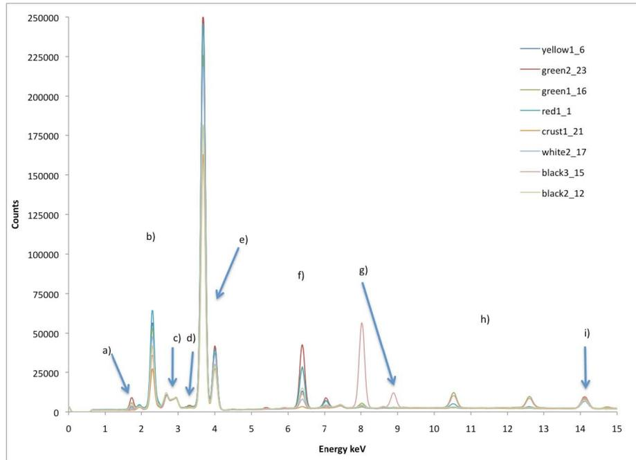
**Fig. 4.** XRF Spectra showing a selected spectrum from each color present. The following peak assignments have been made **a)** Si K $\alpha$ , **b)** S K $\alpha$ , **c)** Rh L (beam), **d)** K K $\alpha$ , **e)** Ca K $\alpha$  and K $\beta$ , **f)** Fe K $\alpha$ , **g)** Cu K $\alpha$  and K $\beta$ , **h)** Pb L, **i)** Sr K $\alpha$ .
