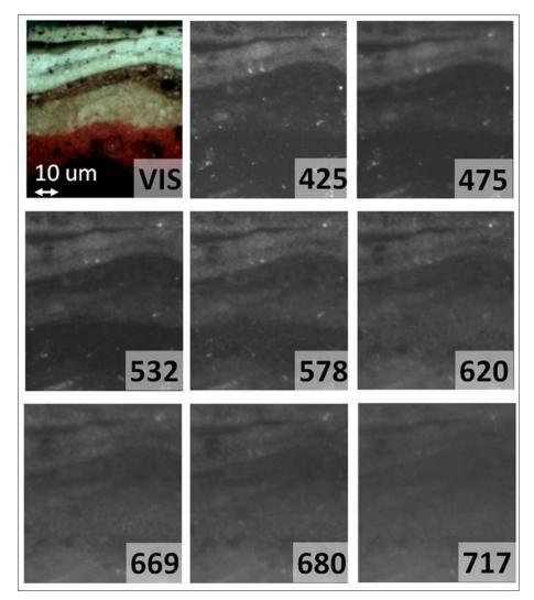
Figure 15: *Madonna and Child*, cross-section, Sampling Point 13 in Figure 14. SpectroCam mounted on a stereomicroscope, RGB image and spectral images.
