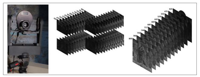
**Figure 3:** Left, SpectroCam mounted on the GigaPan Epic Pro panoramic head. Centre, the spectral images acquired for the four sections of the painting. Right, the stitched, registered and calibrated 12 spectral images of the *Visitation*.
