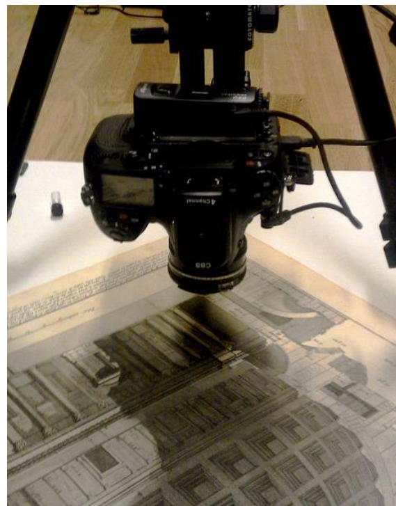
Figure 3. Ingels Collection, Sweden. RTI set up with the camera mounted on macro rail and tripod with reversed tube.
