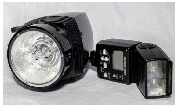
Figure 2. Left: compact and lightweight studio strobe, 180W flash (guide number 45) and 75W modeling bulb. Right: Speedlight Nikon SB-600. This was used for the RTI documentation of the Ingels collection presented in this paper.
