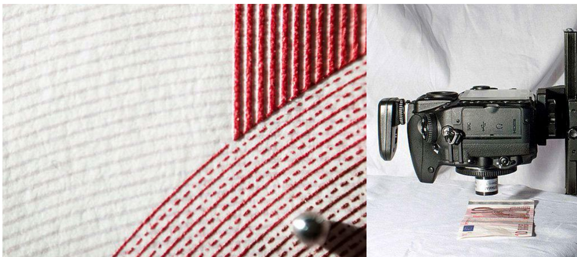
Figure 12. Macro detail of the 10 euro bill (left) and set up (right) with Otamat 2X lens.
