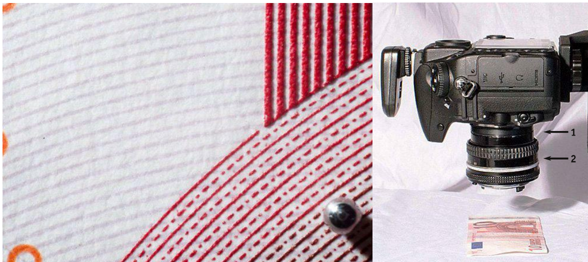
Figure 11. Macro detail of the 10 euro bill (left) and set up (right) with 200 mm lens (1) and reverse ring (2).
