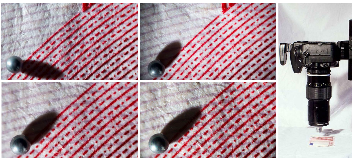
Figure 9. Up to down, left to right: 200mm lens/f8, the sphere is out of focus; 200mm lens/f16, sphere and paper are in focus but vignetting is showing; 300mm lens/f4.5, sphere and paper are in focus without vignetting; 300mm lens/f5.6, sphere and paper are in focus but vignetting is showing. Far right: set up with 200 mm lens, microscope objective adapter and 2X objective.
