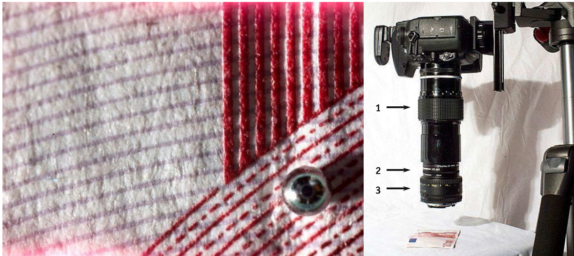
Figure 10. Macro detail of the 10 euro bill (left) and set up (right) with 200 mm lens (1), coupling ring (2) and 50 mm lens.
