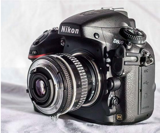
Figure 5. Nikon D800 with some macro set ups. From up to down: reverse ring and 20 mm lens; Otamat Macro Lens; 200 mm lens with Microscope objective adapter and 2X objective.
