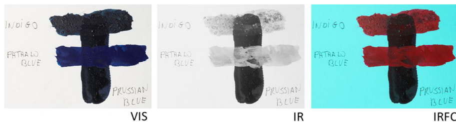
Figure 6 Prussian blue is IR absorbent. In the infrared image phthalo blue appears bright because it is IR reflective. On the other hand, Indigo appears bright because it is IR transparent. Indeed, when it is overlapped with Prussian blue it looks dark. Consequently, the infrared false color of the indigo swatch looks not the ordinary bright red but as dark as Prussian blue.
