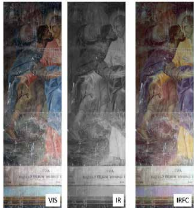
Fig. 8 - The kiss of Judas mural painting. Visible (left) Infrared (middle) and infrared false color (right) images. The red pigment of Jesus' vest strongly reflects infrared, and appears yellow in the IRFC, suggesting vermilion. A cleaning test, visible in the middle of the scene (see dashed line), was administered in order to evaluate both the texture and the state of conservation of the frescoes.
