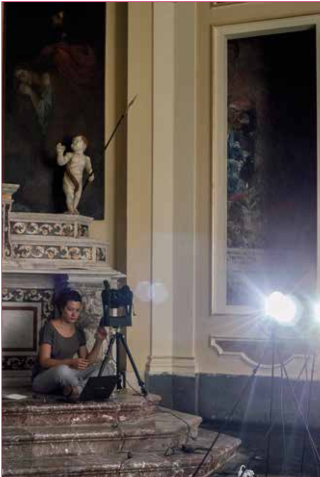
Fig. 4 - The panoramic multispectral imaging system used to document the mural paintings in the Crucifix Chapel.
