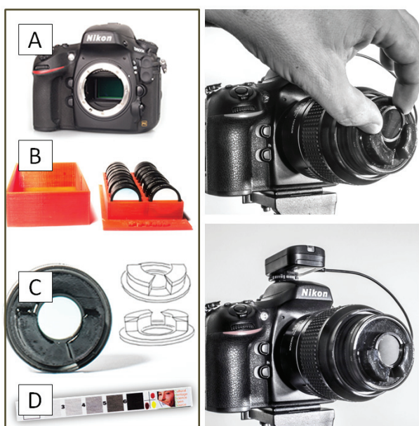
Figure 3. MSI system components. A) Full spectrum modified DSLR camera. B) 18 bandpass filters set. C) Filters adapter. D. In-scene calibration card.
