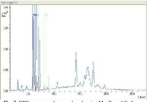
Fig. 5. XRF spectrum of raw umber showing Mn, Fe and Cu lines.
