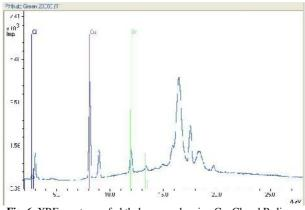
Fig. 6. XRF spectrum of phthalo green showing Cu, Cl and Br lines.
