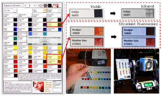
Fig. 1. Pigments Checker. It is designed for pigment identification by imaging and spectroscopic analysis.
