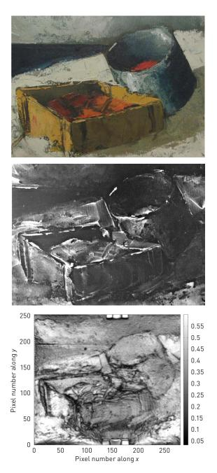
Images of After Fishing, a painting by Ausonio Tanda. (Top) Painting in visible light. (Center) X-ray transmission image of the painting. (Bottom) Terahertz time-domain image, based on raw data. The contrast denotes the peak amplitude of the reflected signal. J. Dong et al., Opt. Express **24**, 26972 (2016)
