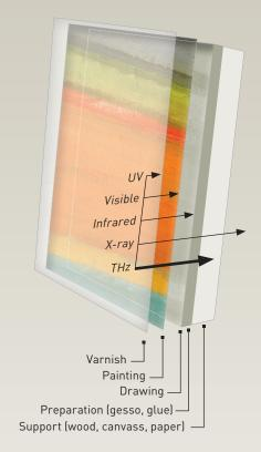
Cross-section of a typical painting, showing the penetration of different types of electromagnetic radiation. Terahertz rays travel farther into the layers than shorter frequencies of light. Although X-rays penetrate artifacts to greater depths, care must be taken with this ionizing radiation.
