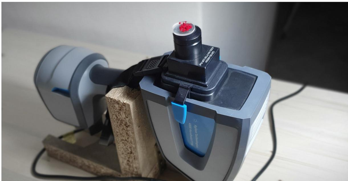
Figure [5]. The IR transparent window holding the powder pigment is loaded on the probe for the spectrum acquisition.
