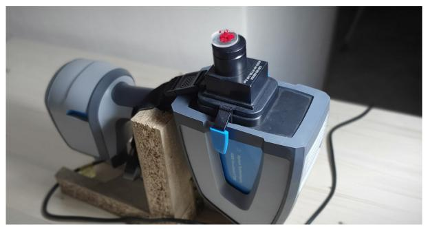
Figure [5]. The IR transparent window holding the powder pigment is loaded on the probe for the spectrum acquisition.
