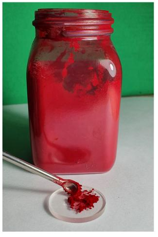
Figure [4]. The powder pigment is deposited on an IR transparent window.
