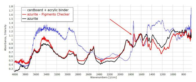
Figure 2. Comparison of the spectra of azurite (pure powder pigment, without any binder); azurite as found in Pigments Checker; the cardboard painted with the acrylic binder. These spectra show that azurite in Pigments Checker show the main features of pure azurite plus the strong peak due to the acrylic binder at 1732 cm -<sup>1</sup>.
