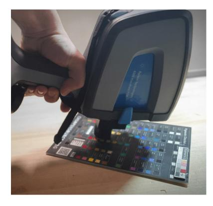
Figure 1. Diffuse Reflectance FTIR analysis on Pigments Checker.
