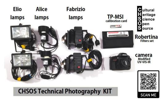
Figure 1. CHSOS Technical Photography KIT. Mandatory components: lamps, camera, filter set, and the calibration card. Optional components are the laptop with pre-installed software, and pigments checker.
