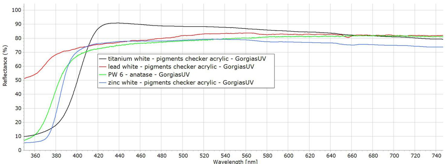
Figure 5. Reflectance Spectra (FORS) acquired with GorgiasUV of the most important historical and modern white pigments.
