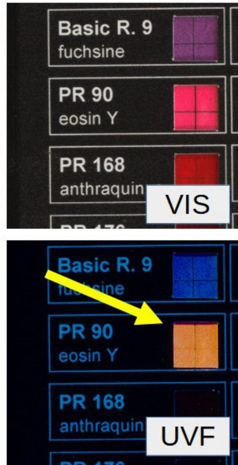
Figure 3. VIS and UVF, detail. PR 90 eosin Y turns from pink to a strong orange.
