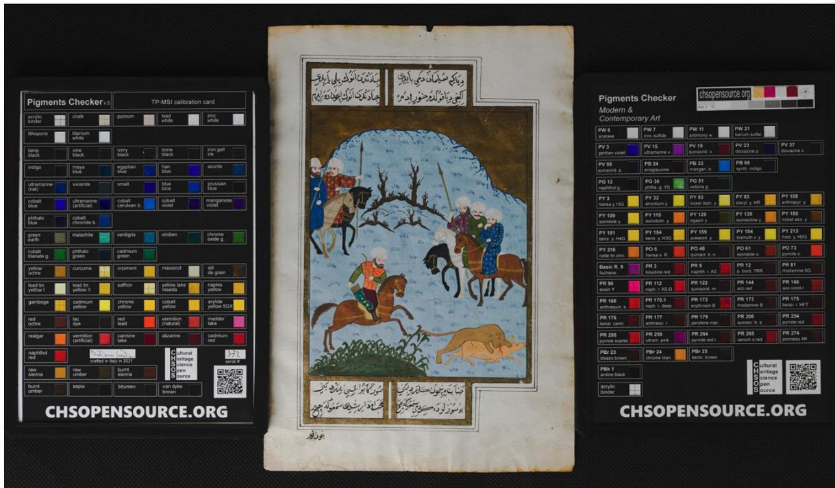
Figure 7. Indian Mughal miniature painting tested with the 2 Pigments Checkers, standard and modern.
