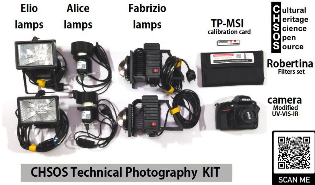
Figure 1. CHSOS Technical Photography KIT. Mandatory components: lamps, camera, filter set, and the calibration card. Optional components are the laptop with pre-installed software, and pigments checker.
