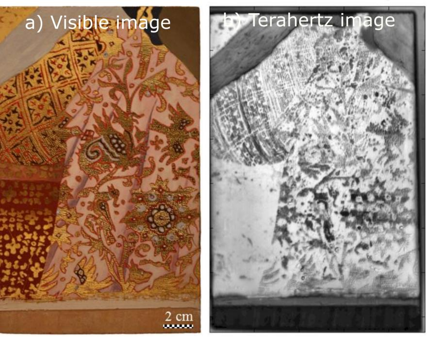
The investigated panel replica n.1 is realized on a wooden support covered by the primer layer. The pictorial scene is complex. The gilding has been used extensively as decorative theme together with the painting material to represent textile. Engravings on the gilding are used to represent geometrical and floral motives.
