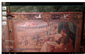
Figure 4. Augmented reality overlay, showing a video see-through representation of a wood panel, augmented with cross-hair markers that are identifying where spectral data was collected.
