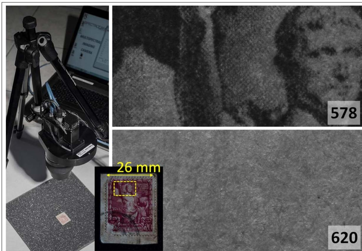
**Figure 11:** Left, SpectroCam equipped with a macro lens (Nikon Nikkor Micro 105 mm f2.8 D). Right, spectral images at 578 nm and 620 nm of the postage stamp in the insert.
