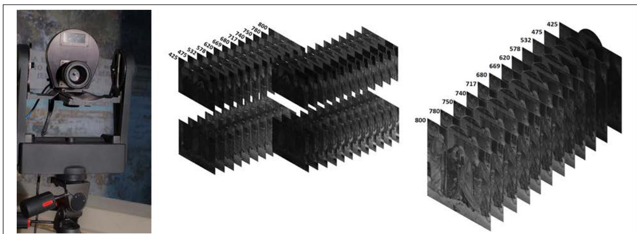
**Figure 3:** Left, SpectroCam mounted on the GigaPan Epic Pro panoramic head. Centre, the spectral images acquired for the four sections of the painting. Right, the stitched, registered and calibrated 12 spectral images of the *Visitation*.
