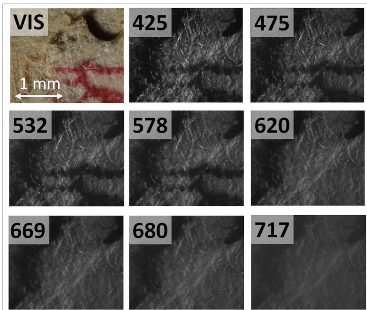
**Figure 17:** SpectroCam mounted on a stereomicroscope. Detail of the postage stamp in Figure 11. RGB image and spectral images.
