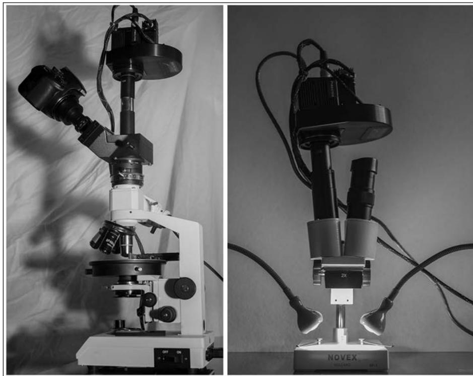
**Figure 13:** Left, SpectroCam coupled with the trinocular head of a compound microscope and a digital camera applied on one of the eyepieces. Right, SpectroCam mounted on one of the eyepieces of a stereomicroscope.
