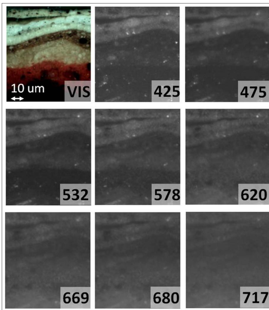
Figure 15: *Madonna and Child*, cross-section, Sampling Point 13 in Figure 14. SpectroCam mounted on a stereomicroscope, RGB image and spectral images.
