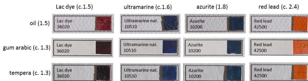
Fig. 3. Examples of pigments and binders with increasing R.I. distances.
