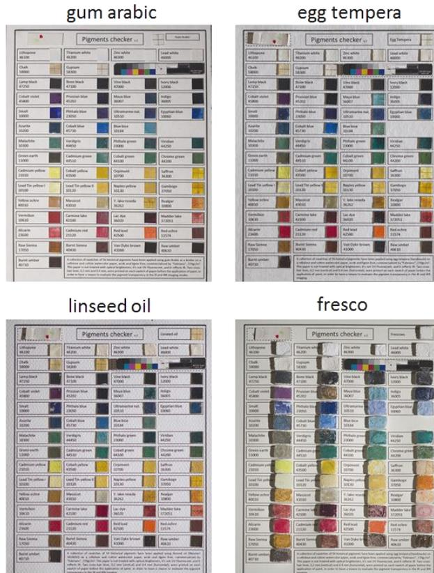
Fig. 1. Pigments checkers. A collection of 54 historical pigments laid with gum arabic, egg tempera, linseed oil and fresco.
