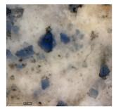
Fig.1. Three images examples of portable digital microscopy for technical studies (x20x) and for diagnosis (smalt pigment at 435x)
