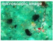
Fig.1: Inclusions of Prussian blue particles in a matrix of emerald green and Arabic gum.
