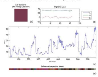
Figure 1 IRFC image for an unknown pigment (a) with Lab parameters (b) and the delta E calculated for every pixel in the reference images (c); the matching color in this case is the second color (d), coresponding to Egyptian blue.
