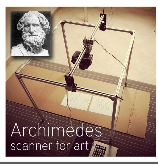
CHSOS has developed <u>Archimedes</u>, the multipurpose scanner for Art Diagnostics. It is a modular low-cost, mobile and lightweight scanner that can accommodate a number of diagnostic imaging methods such as Technical photography, Infrared Reflectography, Multispectral Imaging, and X-Radiography.
