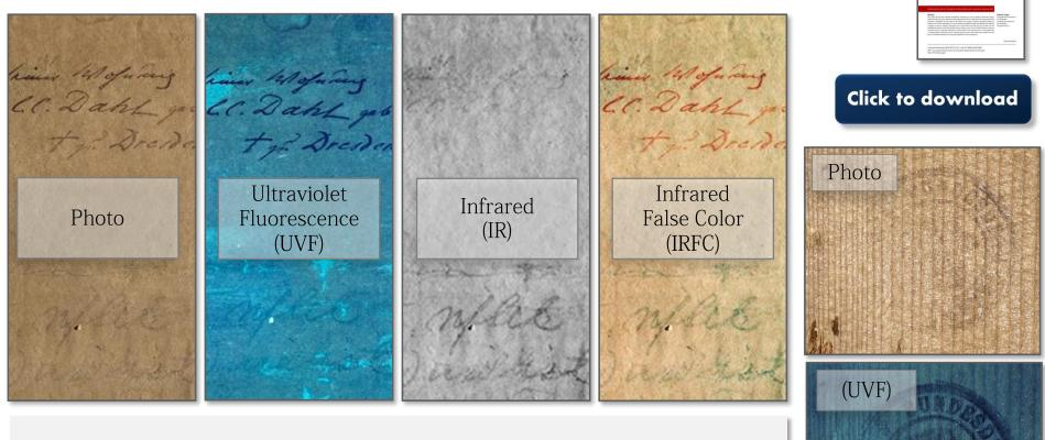
Technical Photography (TP) - a collection of spectral images realized with a modified digital camera and different lighting sources and filters - enhances reading of faded prints, inks, and paints.
