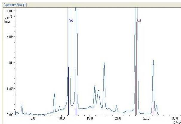
Fig. 7. XRF spectrum of cadmium red showing Cd and Se lines.
