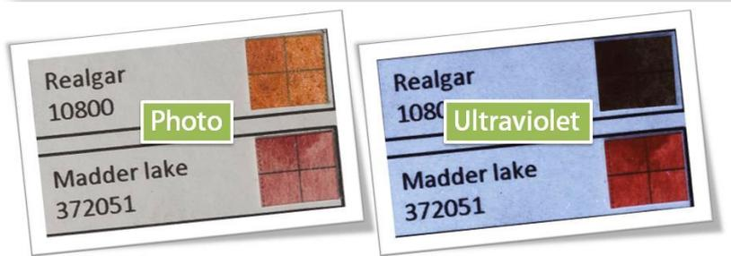
**Swatches:** 2 cross-hairs, 0,2 mm and 0.4 mm printed on each swatch of paper before application of paint, to evaluate pigments' transparency in infrared photography.
