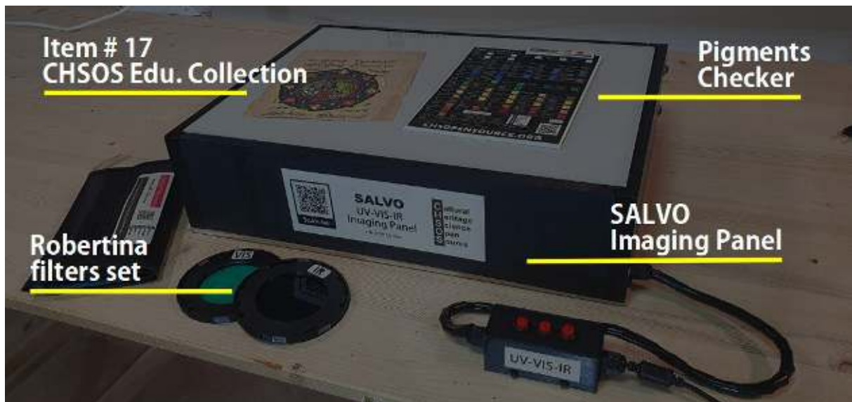
Figure [1]. Some of the equipment used for this application note: SALVO UV-VIS-IR Imaging Panel; ROBERTINA filters set; Pigments Checker; item # 17 CHSOS Educational Collection.
